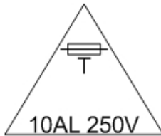
Indicates the Electrical Specification and Location of the Required Fuses
