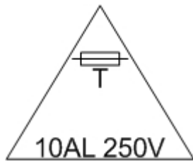
Indicates the Electrical Specification and Location of the Required Fuses
